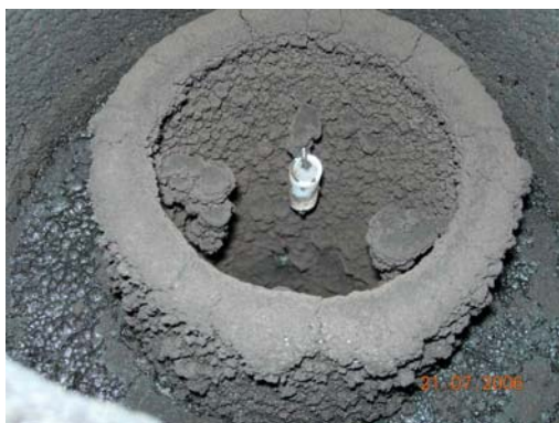
Fig. 1. Carbon steel vessel and coupons collect foulant; FPC coupon (white) remains clean
