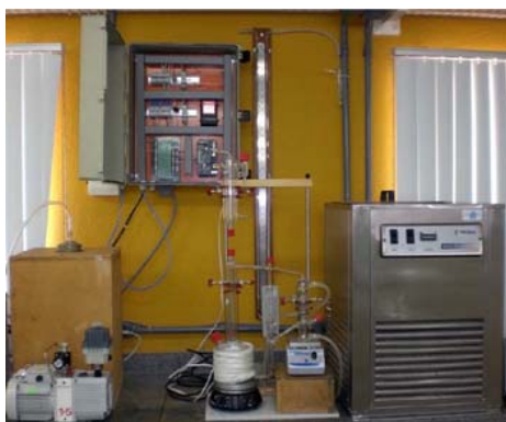
Fig. 1. Vapor-liquid equilibrium apparatus for diluted aqueous mixtures, with organic and salt compounds.
