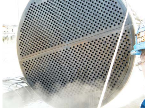
Figure 3 Test exchanger after 6 hours immersion in ultrasonic tank.
