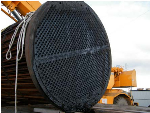
Figure 1 Test heat exchanger bundle prior to cleaning
