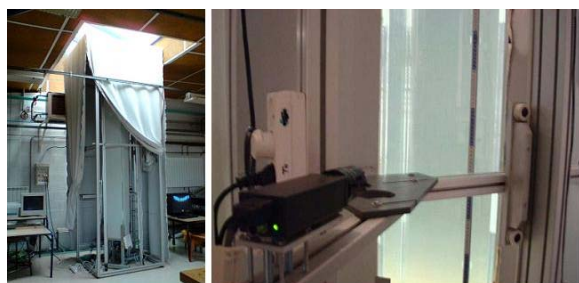
Fig. 1. Rectangular 3 meter high water column, equipped with mobile cameras mounted on a motor
